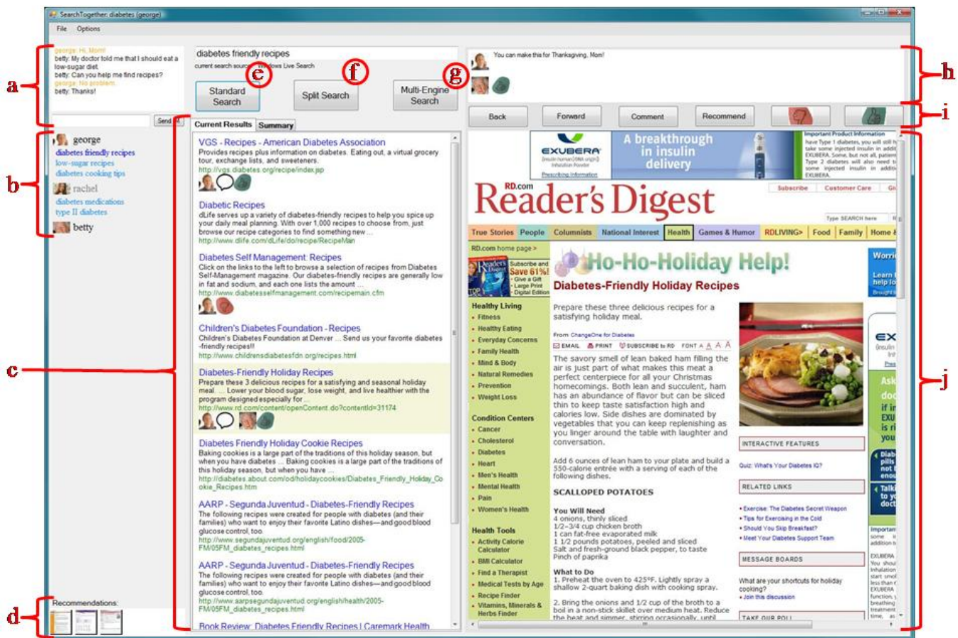
Figure 1. The SearchTogether client. (a) integrating messaging, (b) query awareness, (c) current results, (d) recommendation queue, (e)(f)(g) search buttons, (h) page-specific metadata, (i) toolbar, (j) browser
