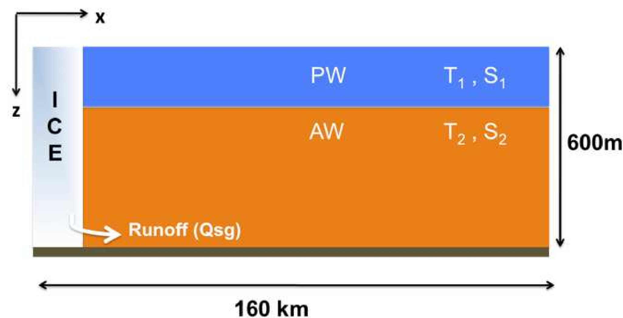
Model geometry with 10m horizontal and vertical resolution. T_1 < T_2 , S_1 < S_2
