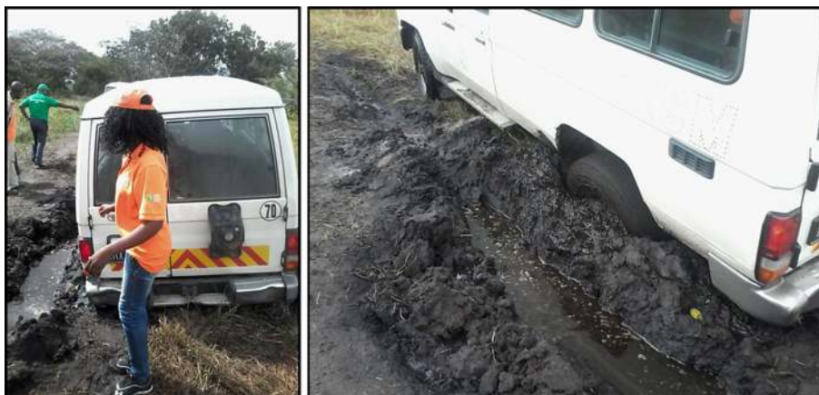
Fig. 4 Illustration of the effect of precipitation on hampering transport on minor unpaved roads—Photo taken by field team during a field visit to Calanga, in Maputo province
