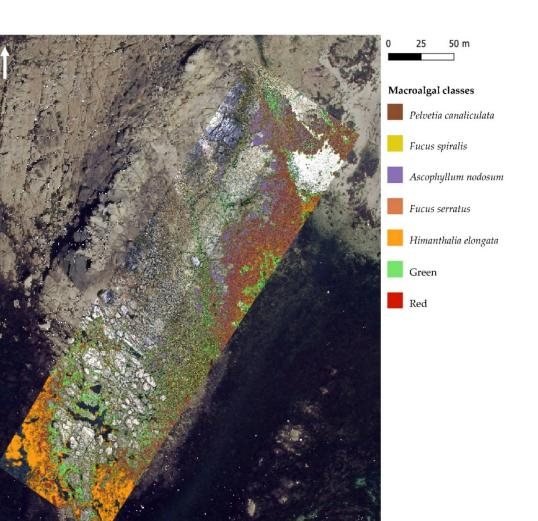
**Figure 8.** Spectral angle mapper (SAM), trained using image-derived spectra resulting from the hyperspectral UAV survey at Porspoder. Seven macroalgal cover classes are displayed over the UAV RGB imagery and an orthophotography (Mégalis Bretagne et collectivités territoriales bretonnes—2015), giving an overview of the site. The 'Substratum' and 'Water' classes are not represented on the map. Class codes 'Green' and 'Red' represent grouped green and red macroalgal species, respectively.
