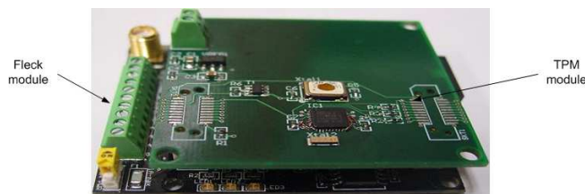
Fig. 2. secFleck (Fleck3 and TPM module).
