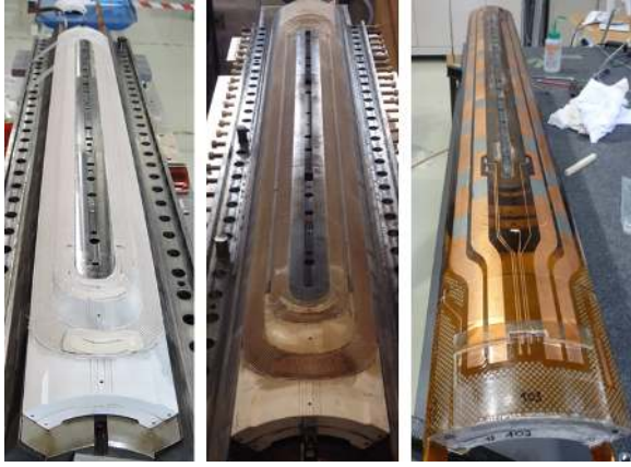
Fig. 1. Coil at different stages of the manufacturing process. From left to right: after curing (2), after reaction (3) and after impregnation (4).
