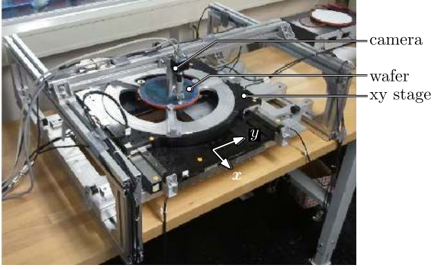
Fig. 5. Industrial application: an xy -wafer stage.
