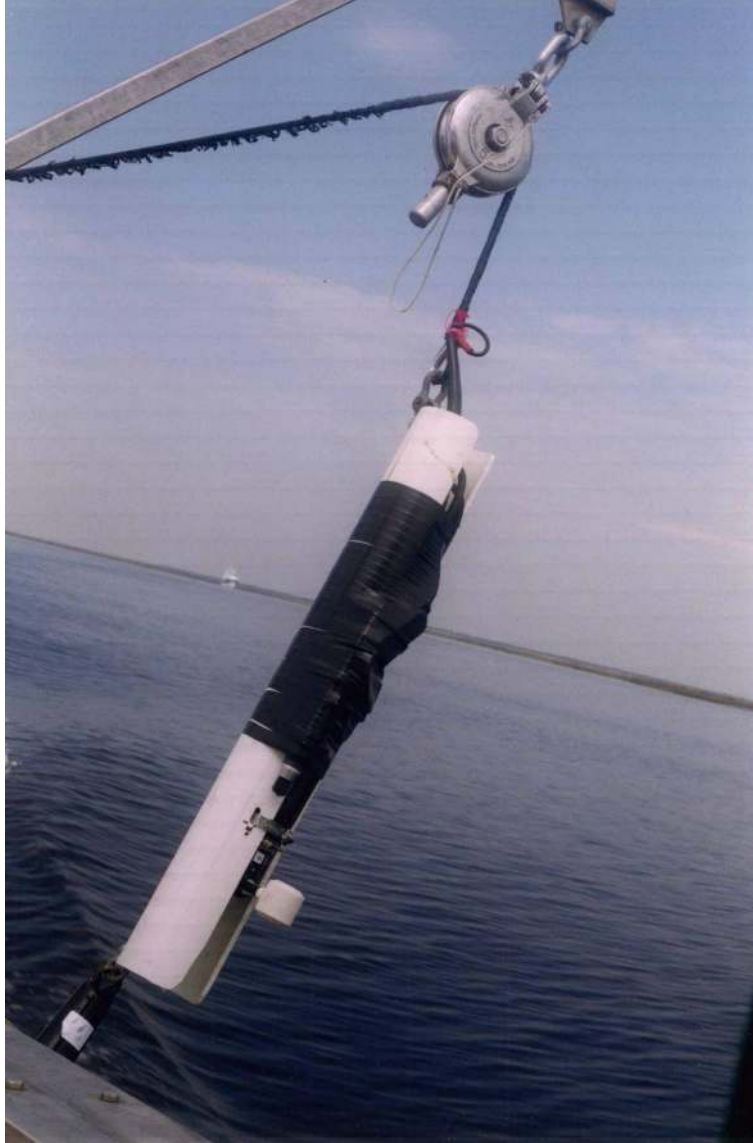
Figure 4.5: A photograph of the Skidaway FSI CTD on the port deck of the R/V Gannet.
