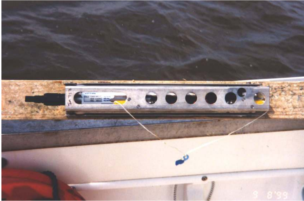
Figure 4.3: A photograph of a Skidaway MicroCAT CTD prior to deployment.
