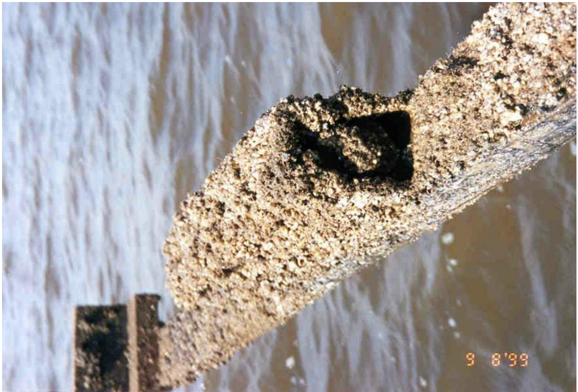
Figure 4.6: A photograph of a Skidaway MicroCAT CTD after a month-long late summer deployment. Rapid bio-fouling occurs when the ambient water temperature exceeds 25°C.
