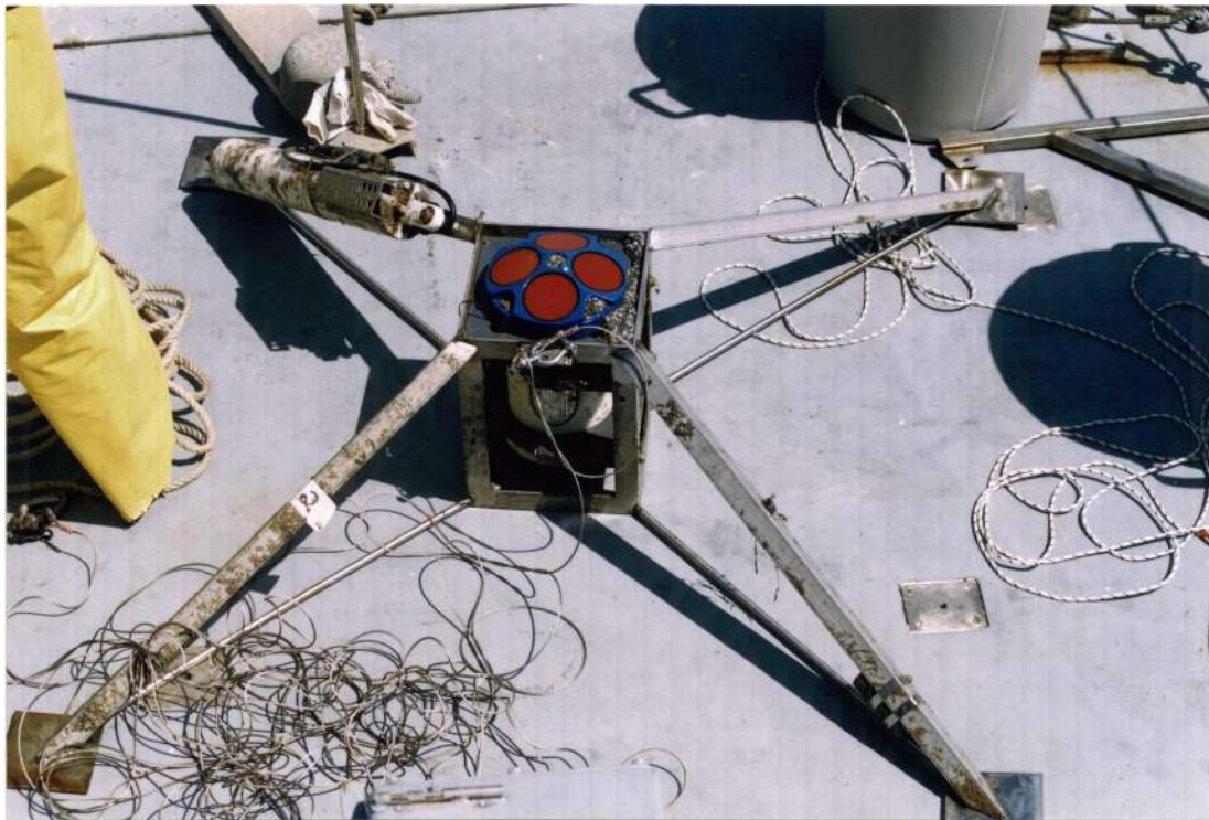
Figure 4.2: A photograph of a Skidaway Work Horse ADCP. A SeaCAT CTD is attached on the upper left leg of the mooring frame.
