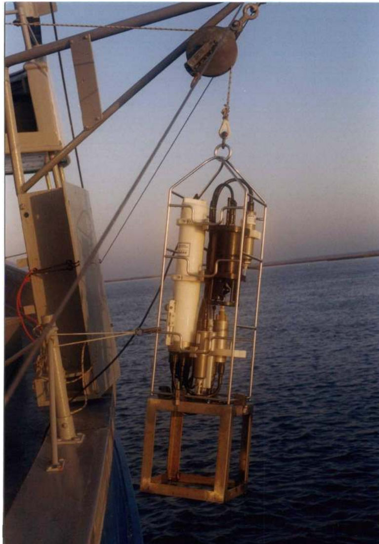
Figure 4.4: A photograph of the Skidaway SBE 19 profiling CTD on the starboard deck of the R/V Blue Fin.
