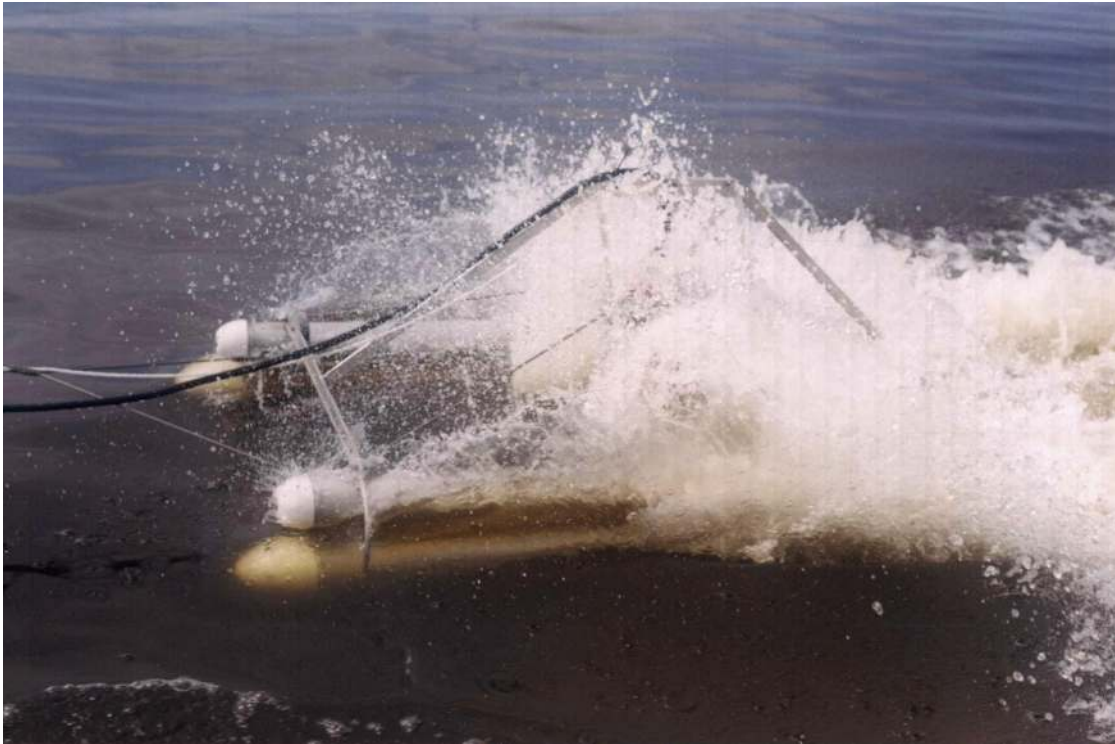
Figure 4.1: A photograph of the Skidaway Broad Band ADCP in tow off the starboard side of the R/V Gannet.
