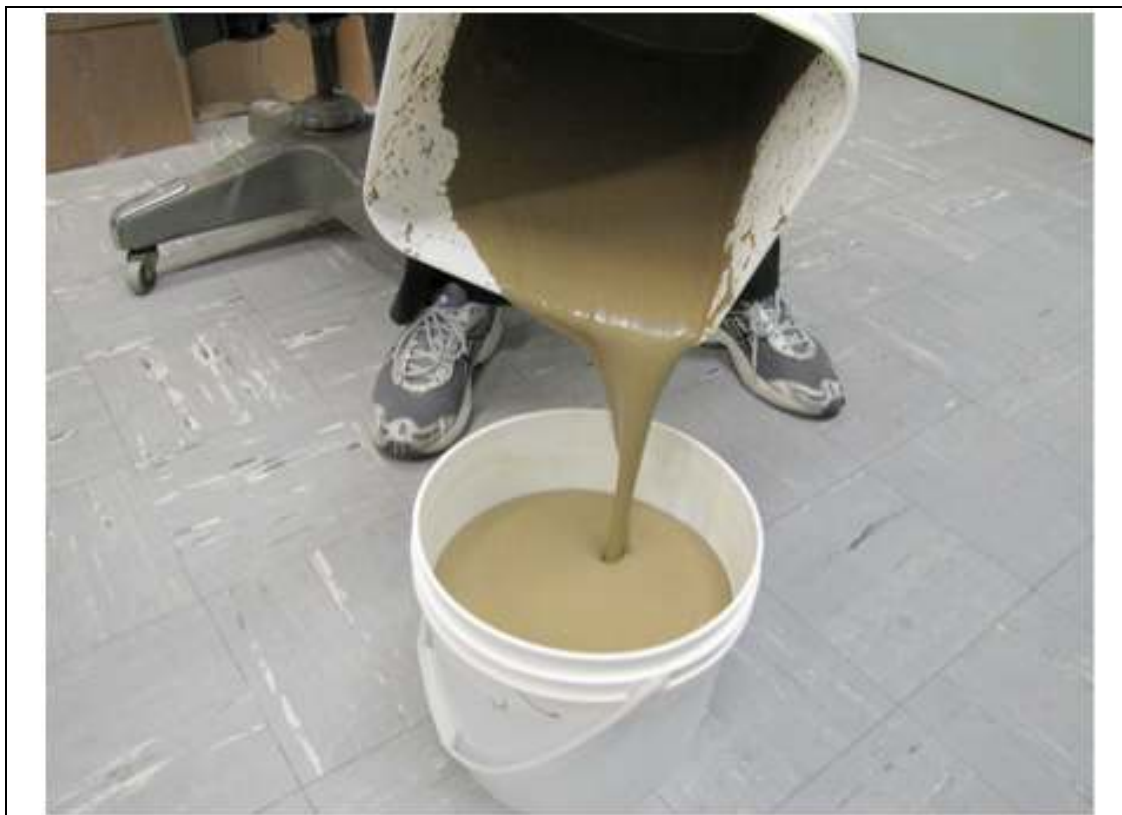
Figure 8-1. Ceramicrete slurry formed during stabilization of baseline waste simulant at 20 wt.% loading
