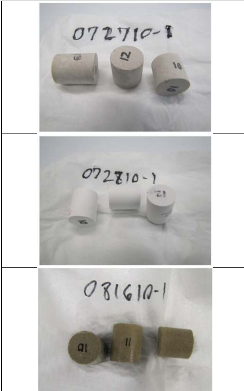
Figure 5-1. Waste form samples with baseline waste simulant loading after 3 months water immersion: (top) 45 % class C fly ash filler +20 % waste, (middle) 45 % \text{CaSiO}_3 filler + 20 % waste, and (bottom) 35% class C fly ash + 10 % slag + 10 % waste
