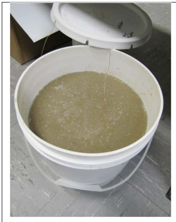
Figure 8-2. Waste form (2 gal) after 3 days of curing
