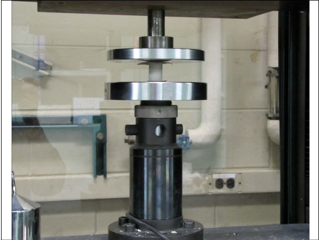
Figure 4-3. Test setup on Instron for measurement of waste form compressive strength
