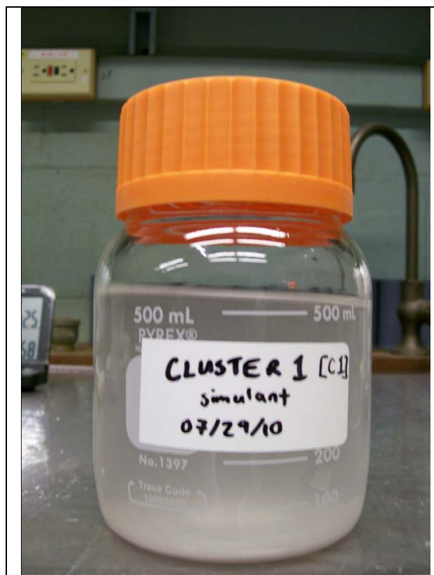
Figure 3-2. Settling of suspended particulates with time in cluster 1 waste simulant
