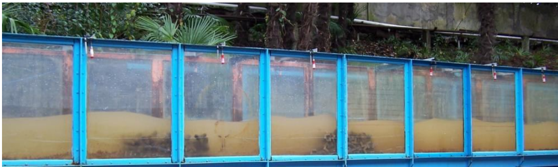
Figure 11. Formation of secondary waves and decreasing of initial wave period after second bar T=1.36 s, H=13.5 cm.
