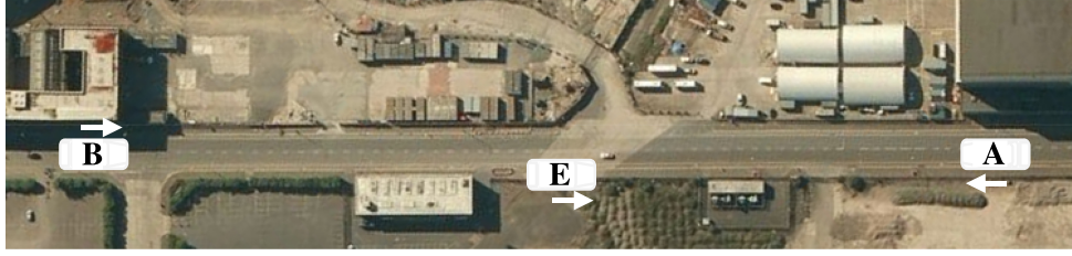
Fig. 10. Satellite view of measurement environment showing the position of nodes A, B and E for V2V scenario. The vehicle with node E remained parked on the side of the road and was oriented such that it faced directly towards node A. Arrows indicate the front of the car.
