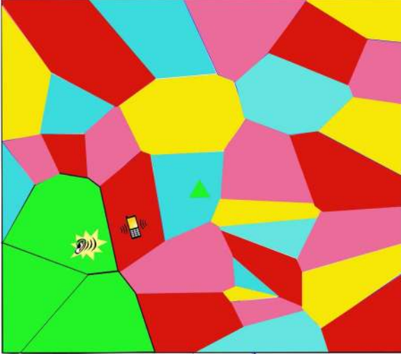
Fig. 2. An example for OSA and SONOSA, where the polygons with the same color denote the femtocells with the same frequency resource, the apple-green triangle is MBS, the cell phone is the eavesdropped MU and the ear denotes the eavesdropper. It is noted that OSA is the underlay strategy, and SONOSA dynamically changes the local pattern of OSA. Three apple-green femtocells are assigned with the same frequency resource as the macrocell to generate CCI against the eavesdropper.
