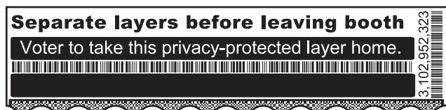
Figure 2. Last inch of the printout before the two laminated layers are separated.
