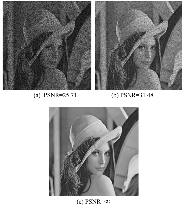
Fig. 4. Images reconstructed in the proposed (2, 4) sharing method with any (k-1) and last share
