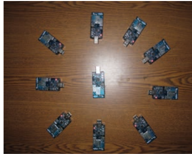
Fig. 9. Experimental setup with ten devices. The central node is designated as the controller. All nodes are displaying synchronous LED blinking patterns.
