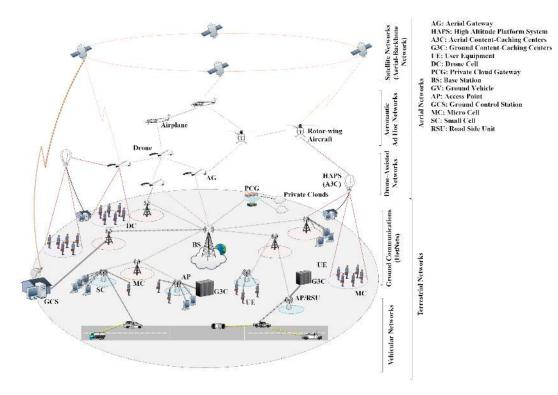
FIGURE 1. An exemplary illustration of ATCNs' architecture, components and dependencies.
