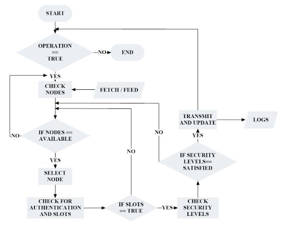
**FIGURE 4.** Cog-chain formation flow chart. The overall approach is demonstrated through the flowchart, which helps to understand the steps to be followed for facilitating cog-chains for secure and reliable content-sharing.
