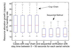
FIGURE 11. Resource allocation growth at 3% request handling rate vs. stay time of an aerial node for cog-chain and sequential-verification method. A: Cog-chain at lower feed time, B: Cog-chain at higher feed time, C: Cog-chain at lower fetch time, D: Cog-chain at higher fetch time, E: Sequential at lower feed time, F: Sequential at higher feed time, G: Sequential at lower fetch time, H: Sequential at higher fetch time.
