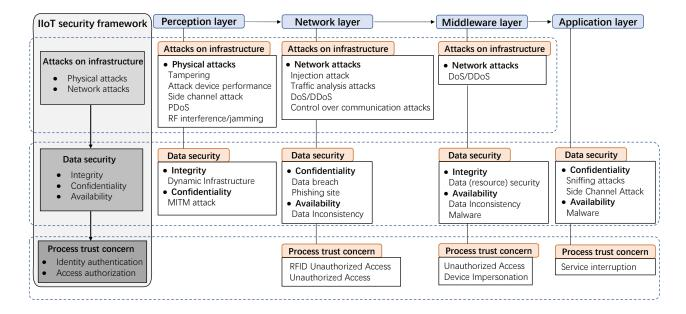
Figure 3. The framework of IIoT security issues.
