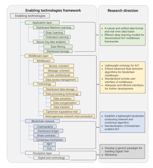
Figure 7. Research direction framework of blockchain middleware for IIoT.
