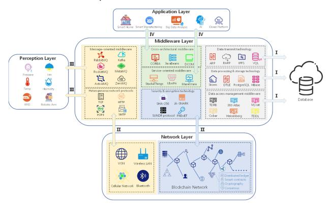
Figure 4. The architecture of the blockchain middleware for decentralized IIoT.
