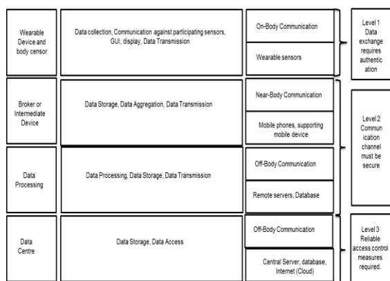
Figure 2. A basic communication architecture for mobile wearables
