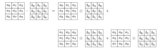
Fig. 1: Our matrix multiplication algorithm with d=3.
