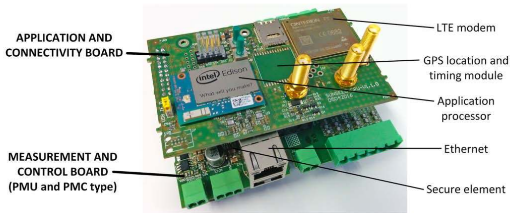
Fig. 1: Illustration of \mu PMU that has been developed for the SUNSEED project.
