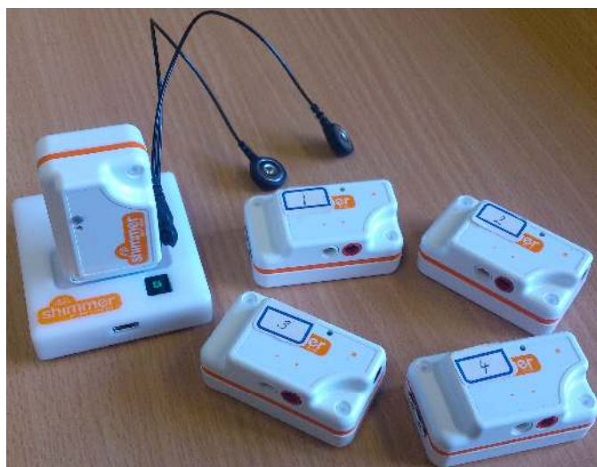
Figure 1. A collection of five Shimmer sensors used to determine the accelerometer bias.
