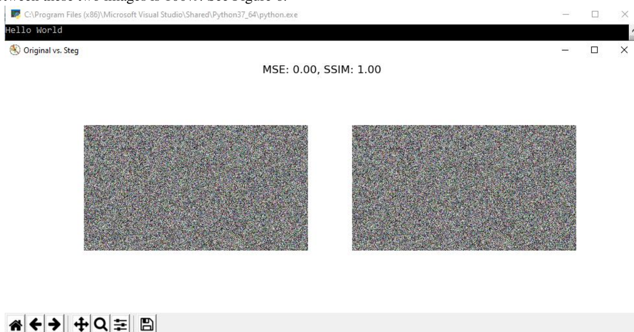
Figure 6. MSE and Similarity between Original Image (Left image) and Steganography image (Right image)
