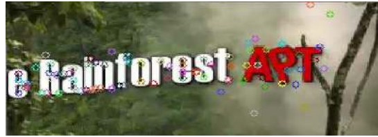
Fig. 4: The circles depict salient features. These salient features are usually corners of an object or texture areas.
