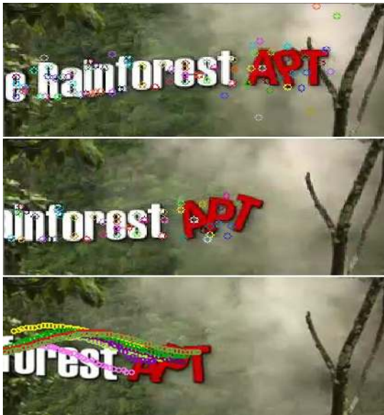
Fig. 5: (Top): salient points in the initial frame. (Middle): salient points with short trajectories in background are discarded. (Lower): trajectories on non-codeword characters are also discarded.
