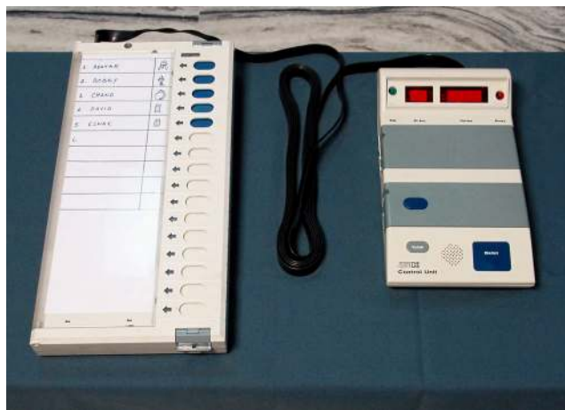
Figure 1: Indian EVMs consist of a BALLOT UNIT used by voters ( left ) and a CONTROL UNIT operated by poll workers ( right ) joined by a 5-meter cable. Voters simply press the button corresponding to the candidate of their choice. We obtained access to this EVM from an anonymous source.
