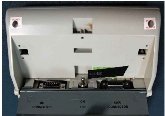
(b) Paper seals (here, broken) cover the screw holes.
