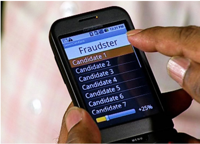
Figure 5: Wireless Signaling — An application running on an Android mobile phone uses Bluetooth to tell our dishonest display which candidate should receive stolen votes. Attacks using other forms of radio communication are also possible.
