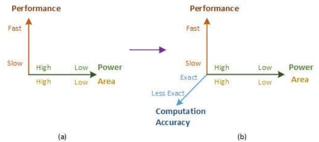
Figure 1: A design space (a) of performance and power for accurate computing (2D) and (b) of performance, power and accuracy for approximate computing (3D).
