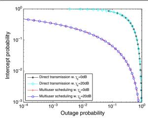
Figure 4 Intercept probability versus outage probability of conventional direct transmission and proposed multiuser scheduling schemes for different  $\gamma_{\rm s}$ . N=8,  $P_{\rm a}=0.8$ ,  $P_{\rm d}=0.9$ ,  $P_{\rm f}=0.1$ ,  $\sigma_{\rm CBS-CU}^2=\sigma_{\rm CBS-CU}^2=1$ ,  $\sigma_{\rm CBS-Eav}^2=\sigma_{\rm PBS-Eav}^2=\sigma_{\rm PBS-CU}^2=\sigma_{\rm PBS-CU}^2=0.5$ , and  $\gamma_{\rm D}=10$  dB.
