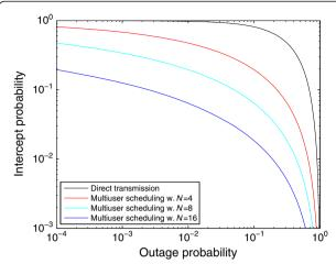
Figure 3 Intercept probability versus outage probability of conventional direct transmission and proposed multiuser scheduling schemes.  $P_{\rm a}=0.8$ ,  $P_{\rm d}=0.9$ ,  $P_{\rm f}=0.1$ ,  $\sigma_{\rm CBS-CU}^2=\sigma_{\rm CBS-CU_i}^2=1$ ,  $\sigma_{\rm CBS-Eav}^2=\sigma_{\rm PBS-CU}^2=\sigma_{\rm PBS-CU_i}^2=0.5$ , and  $\gamma_{\rm s}=\gamma_{\rm p}=10$  dB.
