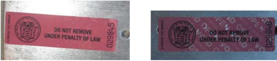
Fig. 13. Pressure-sensitive adhesive tape. At left, as first installed; at right, when (mostly) peeled back and pressed down again.
