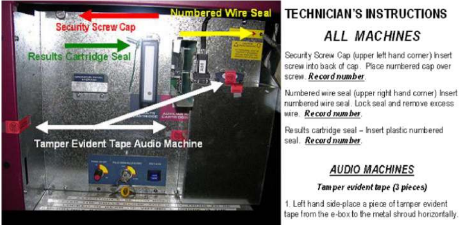
Fig. 10. Sequoia Voting Systems's proposed seal regime, September 2008.
