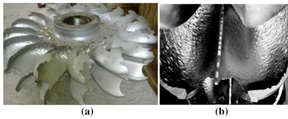
Figure 5 Field erosion of runners in different power stations: (a) Toss HPP, India [8]; (b) Alfalfal HPP, Chile [10]
