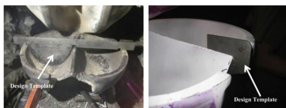
Figure 31 Check the shape of the bucket after maintenance using a template [191]
