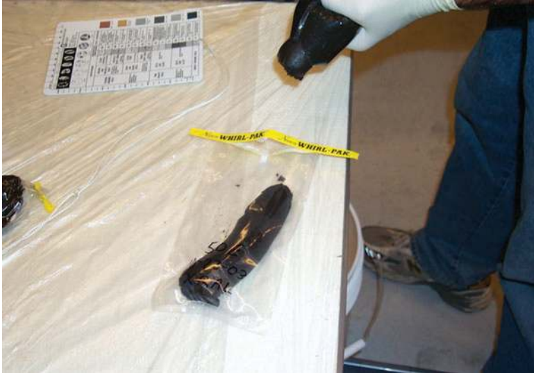
Figure 8. A sample is prepared for metal analysis.
