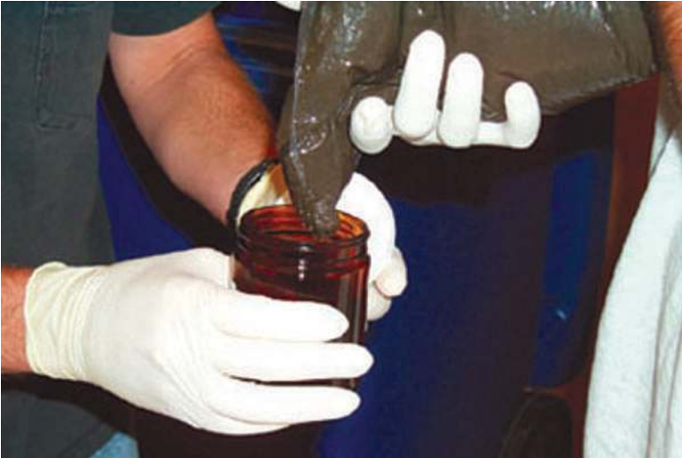
Figure 7. A sample is collected for polychlorinated biphenyl and pesticide analyses.
