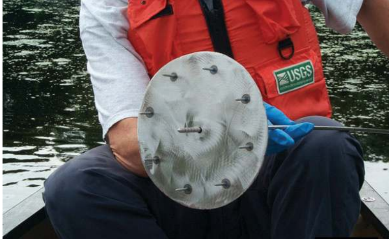
Figure 18. Platform attached to pushpoint sampler in preparation for pore-water sampling. The sampler's screened tip protrudes through a hole in the bottom of the platform.
