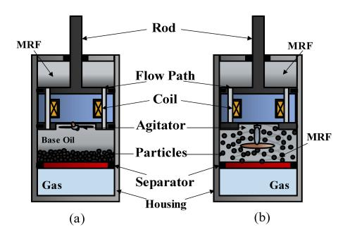
**Figure 7.** Conceptual method to disperse the settled particles in MR damper that has rested for a long time without operation; (**a**) no operation for a long time; (**b**) starting operation after long rest.
