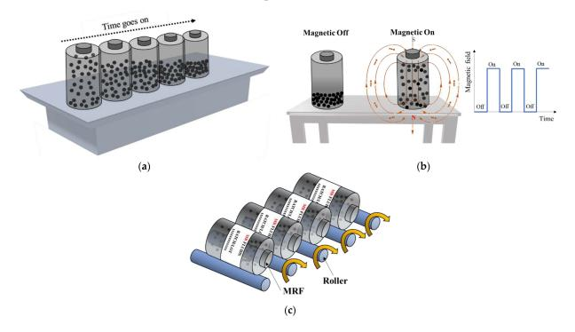
**Figure 6.** Conceptual methods for sedimentation reduction in bottle storage; (**a**) vertical standing on shelf, (**b**) vertical standing with on–off field state, and (**c**) horizontal position in rolling state.
