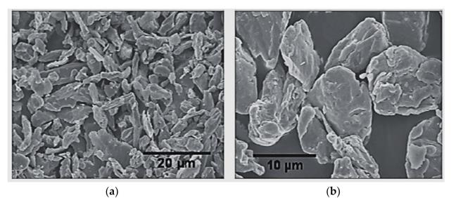
**Figure 2.** Morphology of the microstructure of iron plate-like particles in (**a**) small-sized particles and (**b**) large-sized particles [24].
