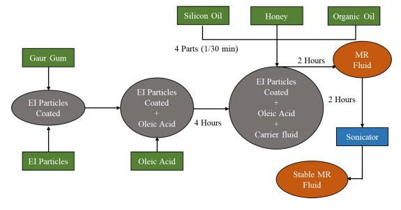
Figure 3. The manufacturing process of magnetorheological fluids featuring various base oils [39].
