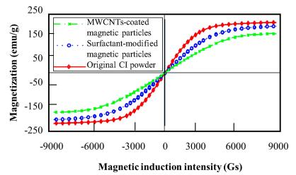
Figure 4. Comparison of magnetization curves of three magnetic particles (1 Gs = 0.0795775 kA = m) [49].
