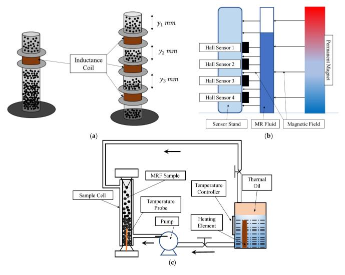
**Figure 5.** Measurement Methods for Sedimentation Rate of MRFs; (**a**) use of inductance coil, (**b**) use of hall sensor, and (**c**) use of thermal conductivity.
