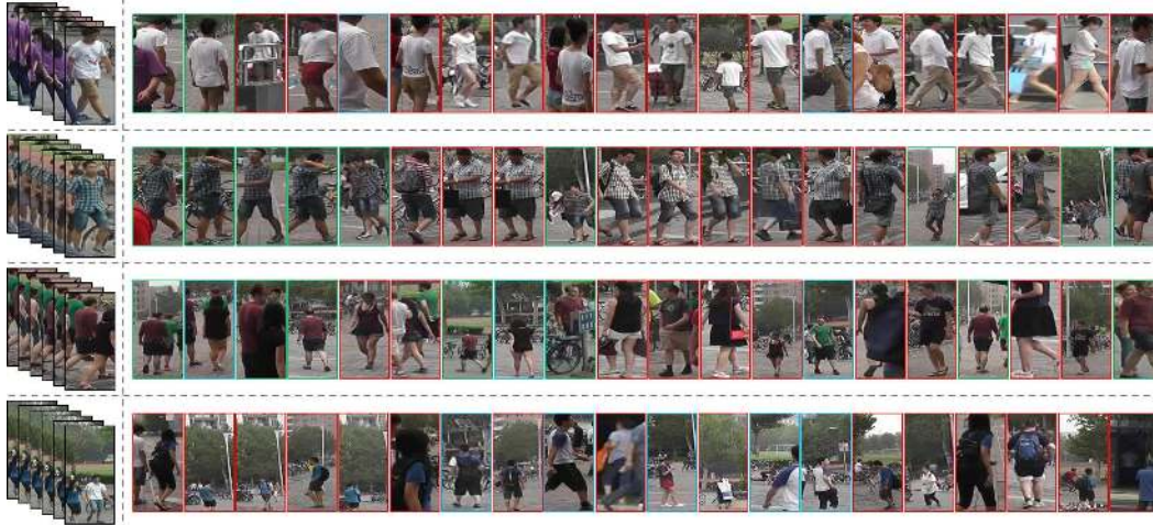
Figure 10: Retrieval results of the proposed method in the testing set of MARS. Image sequences in the first column represent the query. The second column contains candidates in the gallery, where a single image stands for an image sequence for visual-pleasing. Candidates with green boxes indicate that they belong to the same pedestrian as the query. While the red boxes refer to wrong matched image sequences. The images with blue boxes imply that they are distractors, which negatively affect the accuracy.
