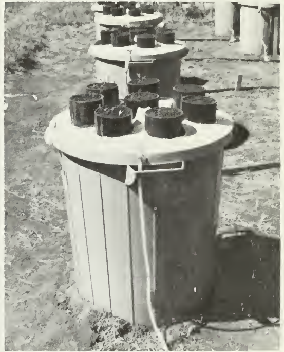
Figure 1.—Refuse barrel with soil-filled pots at beginning of study. Note Tygon tubing and screw clamp used to regulate waterflow.
