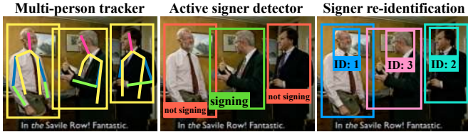
Fig. 2. The SDTRACK framework for diarisation comprises three modules: (left) Multi-person tracker forms person tracks and estimates the pose of each person, (middle) Active signer detector determines which (if any) of the tracked persons are actively signing, (right) Signer re-identification associates identities to each tracked person. See Sec. 3 for more details.
