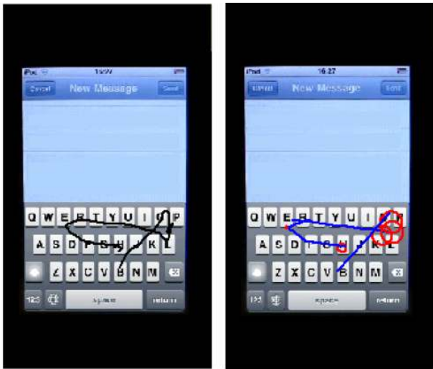
Figure 6: Fingertip trajectory (left) and line modeling (right). The red circles indicate stopping positions for the word “hello”, where the size of the circle corresponds to uncertainty in the stopping position.
