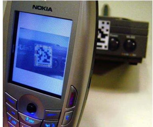
Figure 3 Phone running SiB scanning a barcode on an 802.11 access point (see online version for colours)
