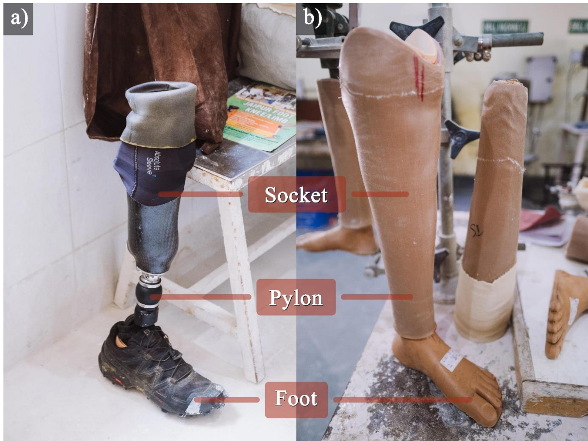
Figure 1: Two lower limb (trans-tibial) prosthetics manufactured using traditional shaping methods. a) The socket on the left is made of a laminated carbon fiber composite which is expensive but common in developed nations. b) The socket on the right is manufactured at a low cost out of high density polyethylene (HDPE) by Jaipur Foot in India
