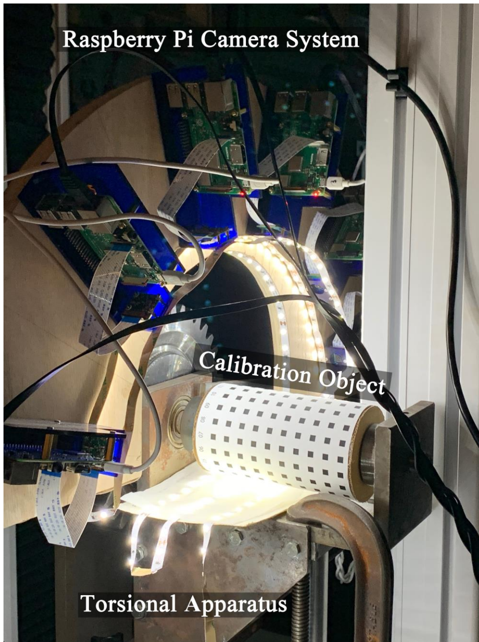
Figure A1: Image showing the assembled 180° synchronized camera array with a precision machined calibration object. This camera array is designed to analyze torsional failure modes in materials.
