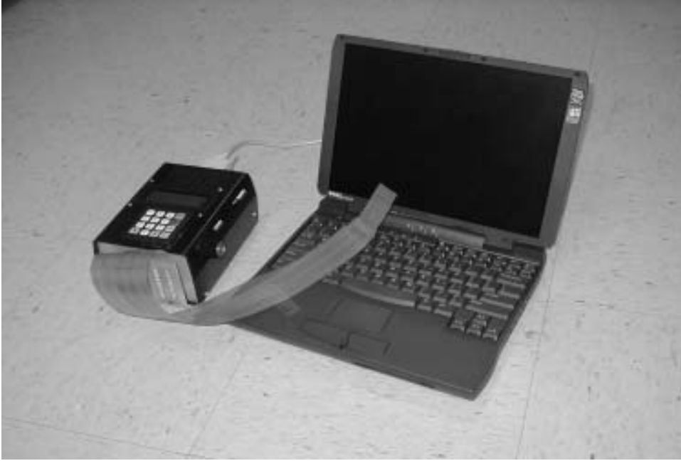
FIGURE 2 TDU-1 with 144-point tongue array & laptop PC.
