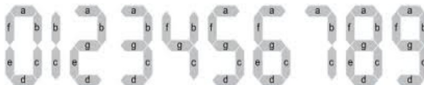
Fig.3: Display of numbers using seven segments
