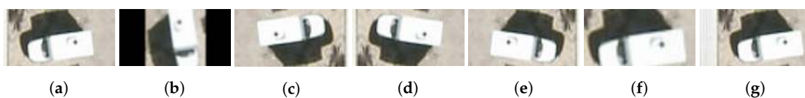
Figure 3. Data augmentation on a vehicle from the VEDAI dataset. (a) original; (b) 90^\circ rotation; (c) 180^\circ rotation; (d) up/down flip; (e) left/right flip; (f) zoom; (g) translation.
