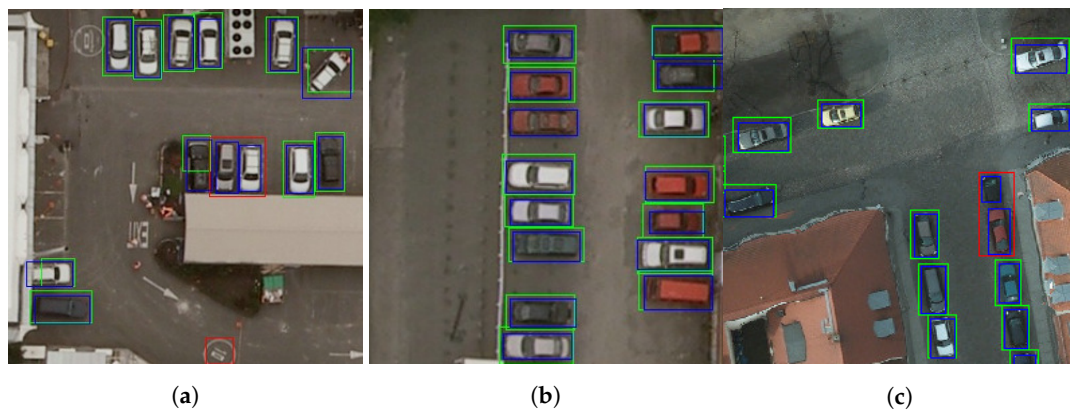
Figure 6. Detection samples on ISPRS Potsdam and NZAM/ONERA Christchurch (true positives are in green, false positives in red and real bounding boxes in blue). (a) vehicle detection on Christchurch; (b) vehicle detection on Christchurch; (c) vehicle detection on Potsdam.
