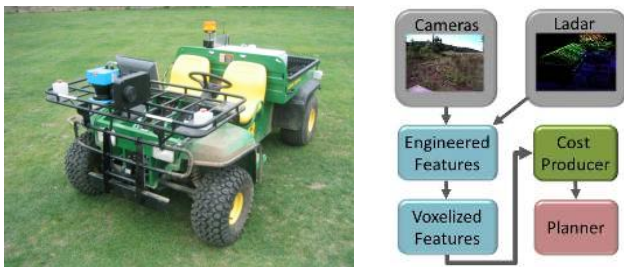
Fig. 4. The E-Gator robotic system (left) and a high-level description of the perception system data flow (right).
