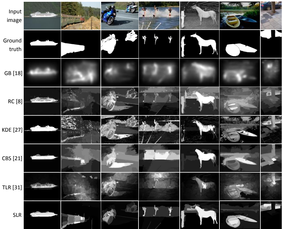
Figure 5: Examples of saliency maps generated using the top 5 models with the best performance in the baselines and the proposed SLR model.
