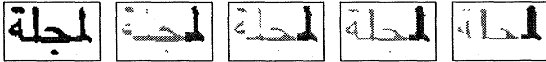
Figure 3: Matching a scanned word with symbol model 1. The left-most image shows the scanned word. The other images, in reading order, correspond to the first four primitives of Figure 5. Each image shows primitives detected on the word in light gray, the correspondence regions of the model in dark gray, and the intersection areas in black.
