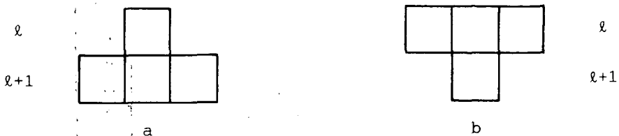
Fig. 3.3. Each hypothesized boundary point has three possible successors (a) and three possible predecessors (b).
