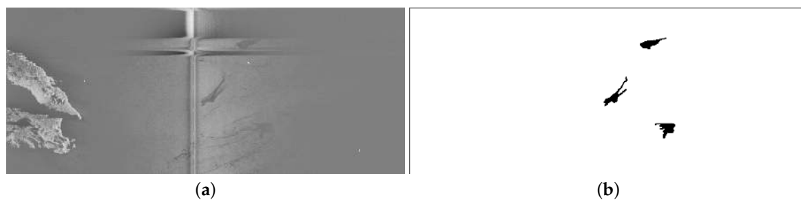
Figure 2. Example of a SLAR sequence from our dataset (a) and its corresponding ground truth (b) with the oil spills labeled at the pixel level. The SLAR image shows an island on the left side, a vertical zone of noise caused by junction of the signal from the two antennas of TERMA radar, and two horizontal bands of noise at the top produced by aircraft maneuvers.
