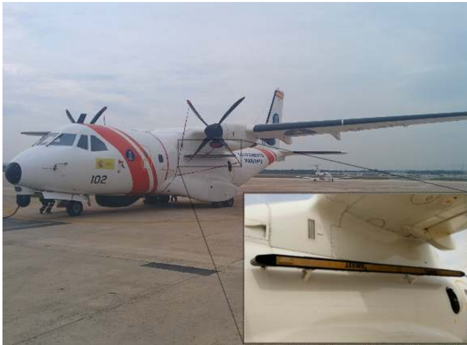
Figure 3. SASEMAR 102 (Variant of CN-235-300 aircraft model for search-and-rescue missions) used to obtain the SLAR sequences, manufactured by EADS-CASA.
