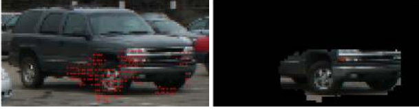
Figure 5. Sparse 3-D points vs. dense image regions. The number of 3-D data points projected on the image is only 193, while MRF labeling delineates the corresponding region with 2007 pixels.
