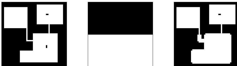
Figure 7.4. Example of conditional dilation; Original image, mask image, and conditionally dilated image.
