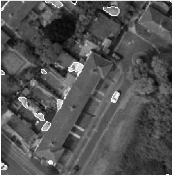
Figure 11. Segmentation result for figure 9 at segmentation scale 20. Segmentation object boundaries are represented by the colour white. Ordnance Survey Crown Copyright. All rights reserved.
