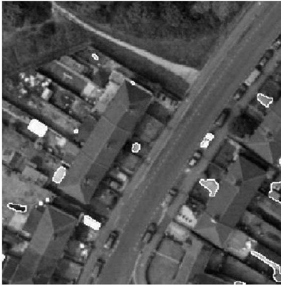
Figure 13. Segmentation result for figure 11(a) at segmentation scale 20. Segmentation object boundaries are represented by the colour white. Ordnance Survey Crown Copyright. All rights reserved.
