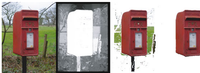
Fig. 1. Example result achieved using the proposed approach. From left to right: original image, saliency map, segmentation by thresholding, and segmentation by using the CRF model.
