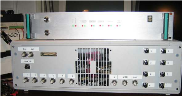
Figure 3: Optoelectronic Piloting Unit, developed by AMS S.p.A. on D'Appolonia design.
