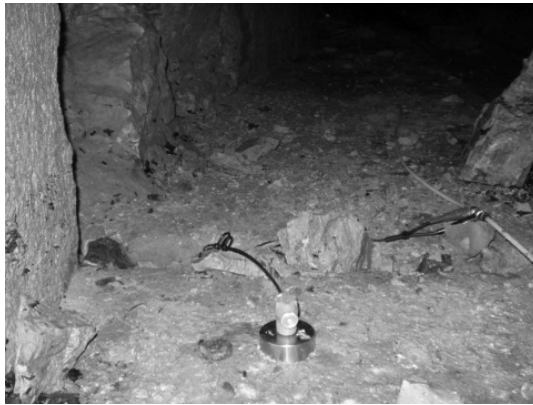
Fig. 3. Deployment of the geophone at the entrance of the mine gallery for the transillumination experiment. The geophone is mounted on a heavy metal cylinder. The cable enters the gallery to reach another geophone at a distance of 5 m.
